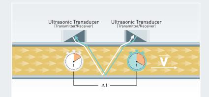
**FLUXUS® F601** is available in three versions: Standard, Energy, and Multifunctional. These versions differ in their equipment with signal inputs and outputs (see table below). The transducers need to be selected according to the application. Transducers are available for a diameter range from DN 6 to DN 6500 and for temperatures from -40 °C to 400 °C.
