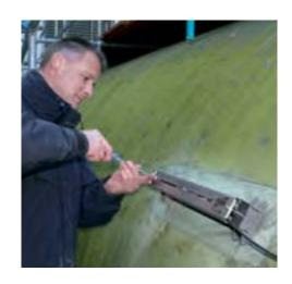
VARIOFIX L is the standard transducer mounting fixture and VARIOFIX C provides optimum protection even in the harshest conditions: beneath the stainless steel cover, the measuring point is permanently protected against external influences, wind and weather as well as mechanical damage.
