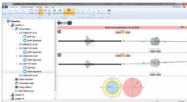
Detailed view of coupling and foot values, including axial view in the result screen
