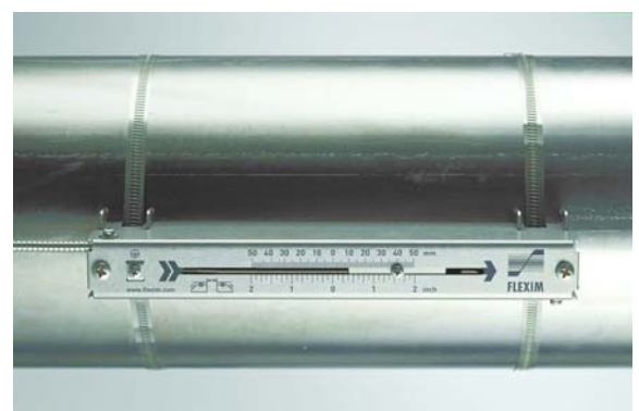
Measurement with transducers mounted by Variofix L
