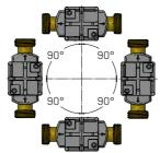
The flow sensor can be mounted horizontally, vertically or at an angle.
