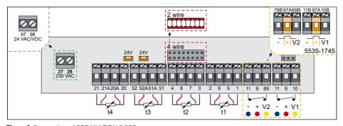
Figure 1 Conncetion of PCB MULTICAL® 803
