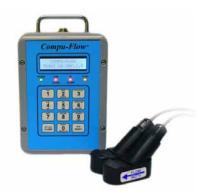
Doppler ultrasonic flow meters provide an accurate and easy-to-use measuring system for high-solid fluid flow through pipes 0.50 inch to 999 inches (inside diameter). The Doppler flow meter is well suited for flow measurement applications such as sludges, slurries, aerated liquids, sewage, dredges, pulp, plastics, and activated sludges. It measures flow velocity by sensing signals from reflective materials within a liquid flowing in the pipe.
